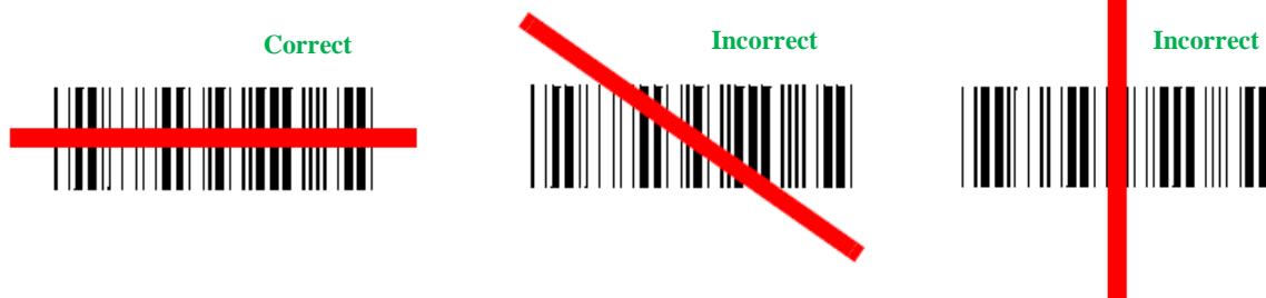
Figure 1: Correct and incorrect scanning
